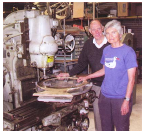
Fig. 7. Machining the one of the flat surfaces of the meridian ring. Further work follows for the displaced circular outlines of the ring.
