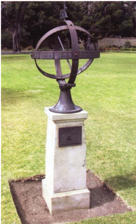
Fig. 5. An earlier design of armillary that has a uniform equatorial ring. Attractive features are the banner on the top and signs of the zodiac on the horizon ring. Sadly the tip and fletching of the gnomon 'arrow' have recently been cut off for safety reasons, but it is said that the lawns are used for many social functions.
