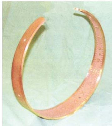
Fig. 8. An hour ring after rolling into shape.
